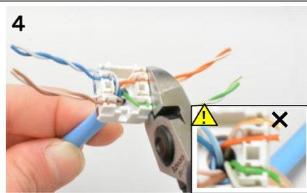
◆ Cut the extra insulation at the end of the cap.
