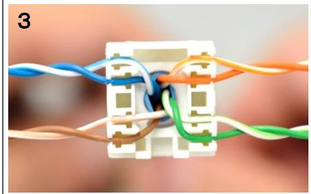
◆ Line up according to the wiring label.
