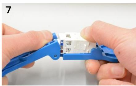
◆ Using the principle of leverage, fit the wire cap and the body.
