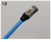
◆Removed from crimping tool, assembly is complete.
