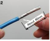
◆Remove the cable jacket about 40mm. and remove the polyester tape.
