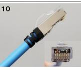
◆Make sure that the core wire reaches the tip of the plug housing and that there is no gap between the boot and the plug housing.
