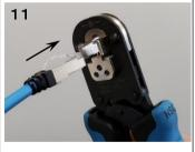
◆Using the crimping tool NST88, insert the plug securely into the tool and crimp it.
