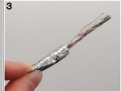
◆Fold back the shielding tape.
